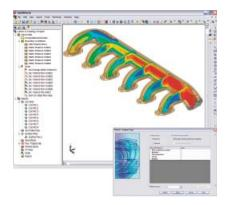
COMOSFloWorks powerful wizard based user interface and goal based flow analysis makes it easy for you to perform flow analysis on virtually any SolidWorks model, like this exhaust manifold. Understanding how much gas moves through each individual outlet of the manifold allows you to make design modification in order to attain specific design criteria.
