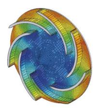
Identify structural failures that can occur due to fluid pressure regions by combining the analysis power of COSMOSFloWorks and COSMOSWorks®. Plot the pressure distribution profile in COSMOSFloWorks and easily transfer these pressures to COSMOSWorks to perform a stress analysis.
