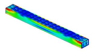
Cargo Ship Linear Static Analysis: 10,963,000 DOF. Total Solution time: 3.58 hr. Run on an Intel Itanium 2 1.0 Ghz CPU with 6GB of RAM in 64-bit NEi Nastran for Linux.
