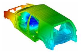
SUV Modal Analysis: 1,230,000 DOF. Total Solution time: 30.5 min. (20 modes) and 66.6 min. (100 modes). Run on a dual Intel Xeon + 3.2GHz CPU with 3GB of RAM.
