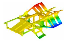
Modal Frequency Response Analysis of an Automotive Frame: 3,163,596 DOF. Total Solution time: 3.2 hr. (75 modes) and 7.5 hr. (150 modes). Run on a dual Intel Xeon + 3.2 GHz CPU with 3GB of RAM.
