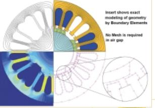
Angular periodic model of a permanent magnet motor.
