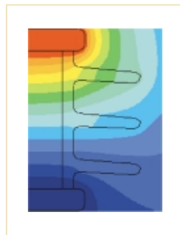
Voltage contour plot of high voltage insulator
