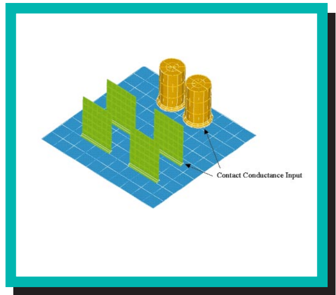
Contact conductance between non-aligned edges/areas automatically calculated
